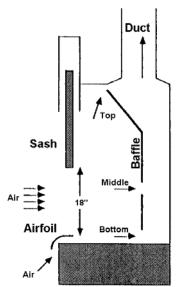
Figure showing common baffle locations
